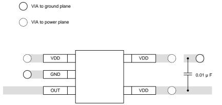
Figure 19. SC70 Package Recommended Layout
