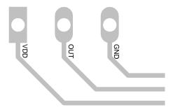
Figure 21. TO-92 LPM Package Recommended Layout
