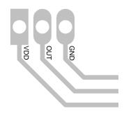
Figure 20. TO-92 LP Package Recommended Layout
